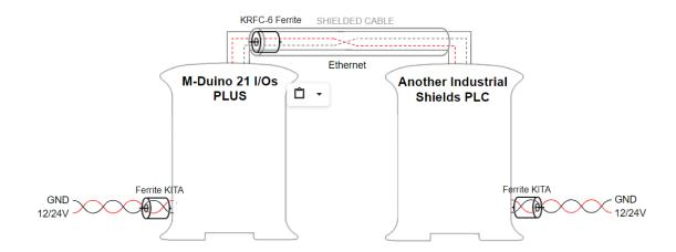
For Ethernet communication between Industrial Shields equipment a **SFTP CAT-6 Ethernet crossover cable** must be used.
