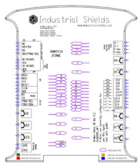
HS\*: Hardware Serial HD\*: Half Duplex SS\*: Software Serial FD\*: Full Duplex
