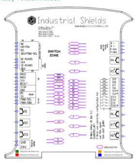
HS\*: Hardware Serial SS\*: Software Serial HD∗: Half Duplex FD\*: Full Duplex
