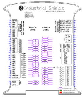
HS\*: Hardware Serial SS\*: Software Serial HD∗: Half Duplex FD\*: Full Duplex
