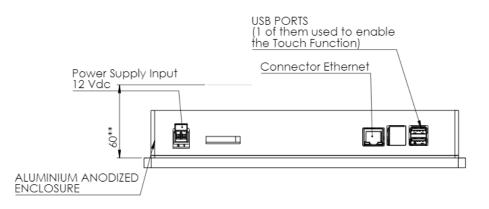
Ethernet and USB port connectors (One of the USB ports is connected in order to activate the attach function)
