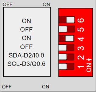
\*I2C switch serigraphy is turned around. It should be: (SDA-D2 , SCL-D3). RX-RS485 should be RE-RS485
